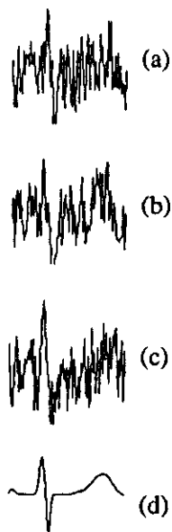
Figure 9.4 Summing the time-aligned signal epochs corrupted with random noise such as those in (a), (b), and (c), which were extracted from Figure 9.3, improves the signal-to-noise ratio. The result of averaging 100 of these ECG time epochs to improve the SNR by 10 is in (d).
